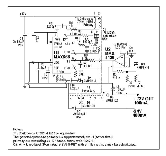
This circuit uses the MAX668 and a transformer (which will need about a 1:2:2:2 turns ratio) to make a flyback converter. The op amp inverts the feedback from both negative output voltages.
